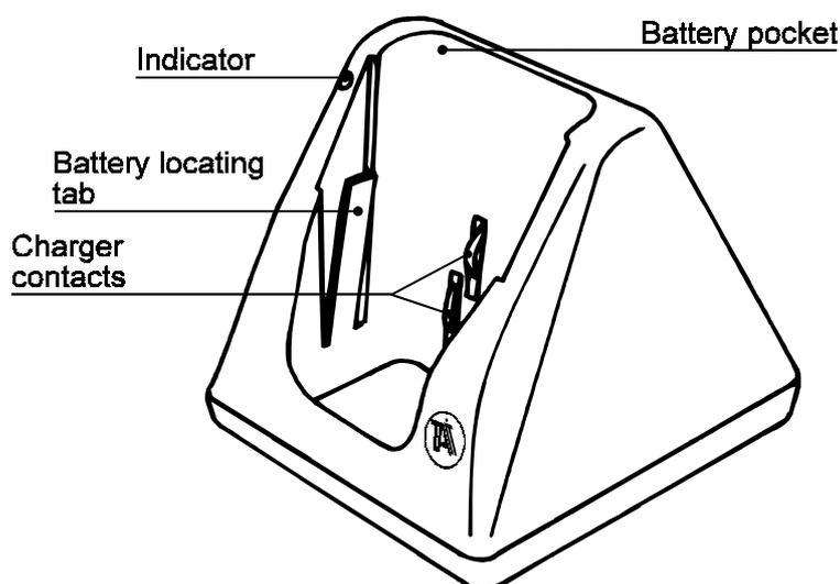
The T3003 desktop trickle charger is designed to charge T3000 rechargeable battery packs, with one slot for either the combined battery and radio or for the battery alone. The charger is powered by either a dedicated T952 AC/DC plug pack, complying with the local requirements of the country into which it is sold, or a suitable DC supply. A dual coloured red and green LED displays the charge status of the battery.
